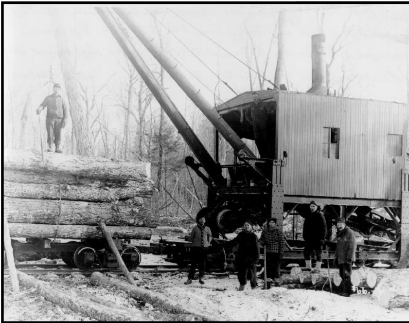
The above picture shows a Skeleton Log car at the VCLCo. It has been suggested this car was manufactured by the Russel Wheel & Foundry Co. of Detroit, MI.
