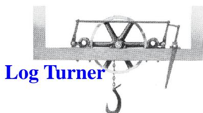
The turning of logs on the Carriage was normally done by manual labor, several workmen with cant hooks or peavies being required to turn a log for sawing. To increase the daily capacity of Sawmills, the hand operation was discontinued and replaced by a powered device.
